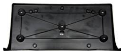
Fig.3b Real part warpage
