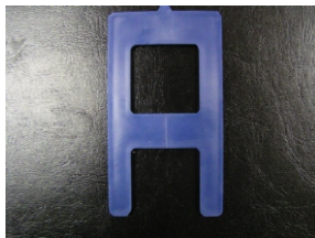
Fig.4(a) Weld line formed by cold melt which results in brittle fracture
