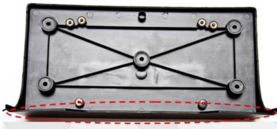
Fig.1 The warped part after first sampling
